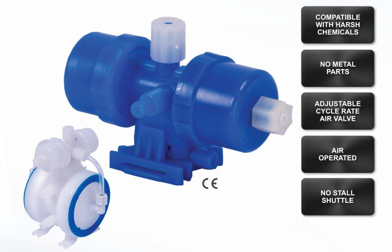
The PC7 operates as a single valve oscillator to switch the air supply pressure and exhaust for a pneumatic pump. It was designed with our no stall shuttle so the value is always cycling. The cycle rate is controlled by a combination of air supply pressure and detent force, which is adjustable.
