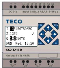
**Figure 8: Remote Mode (ON)**
