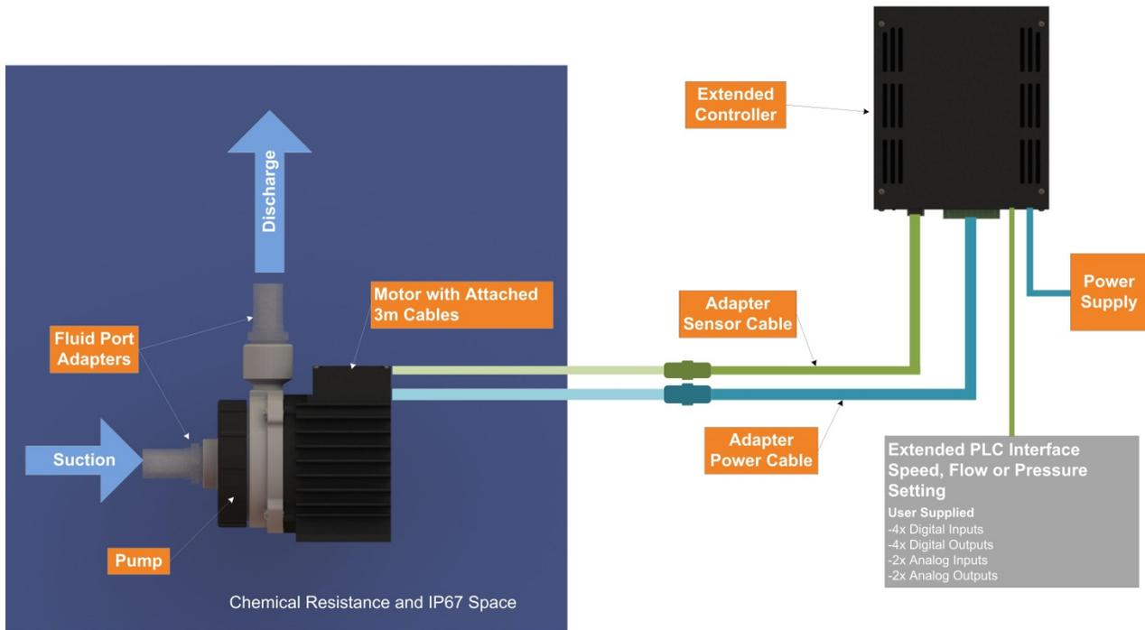
**Figure 3 – Extended System Configuration for Extended Control (Rev6A1)**
