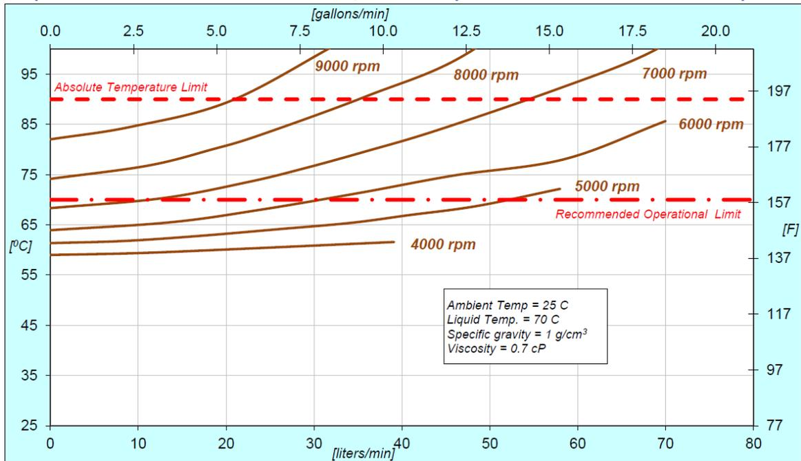
Figure 17 - Temperature curves of the Motor for 70°C Fluid Temperature
