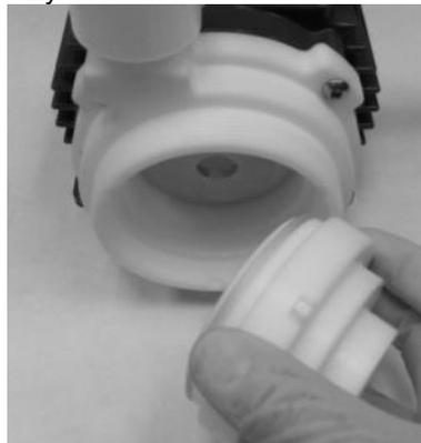
9. Carefully tighten the union nut. Tighten by hand until the union nut is flush with the surface of the inlet housing. Add an additional 1/8 turn or 8-9 Nm (70-80 in-lbs.) of torque.
