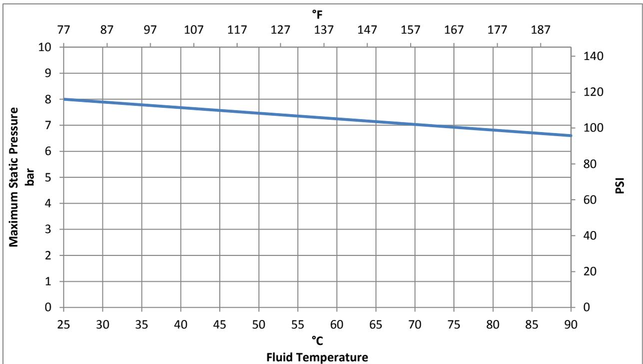
Figure 6 – Maximum Static Pressure Allowed vs. Fluid Temperature
