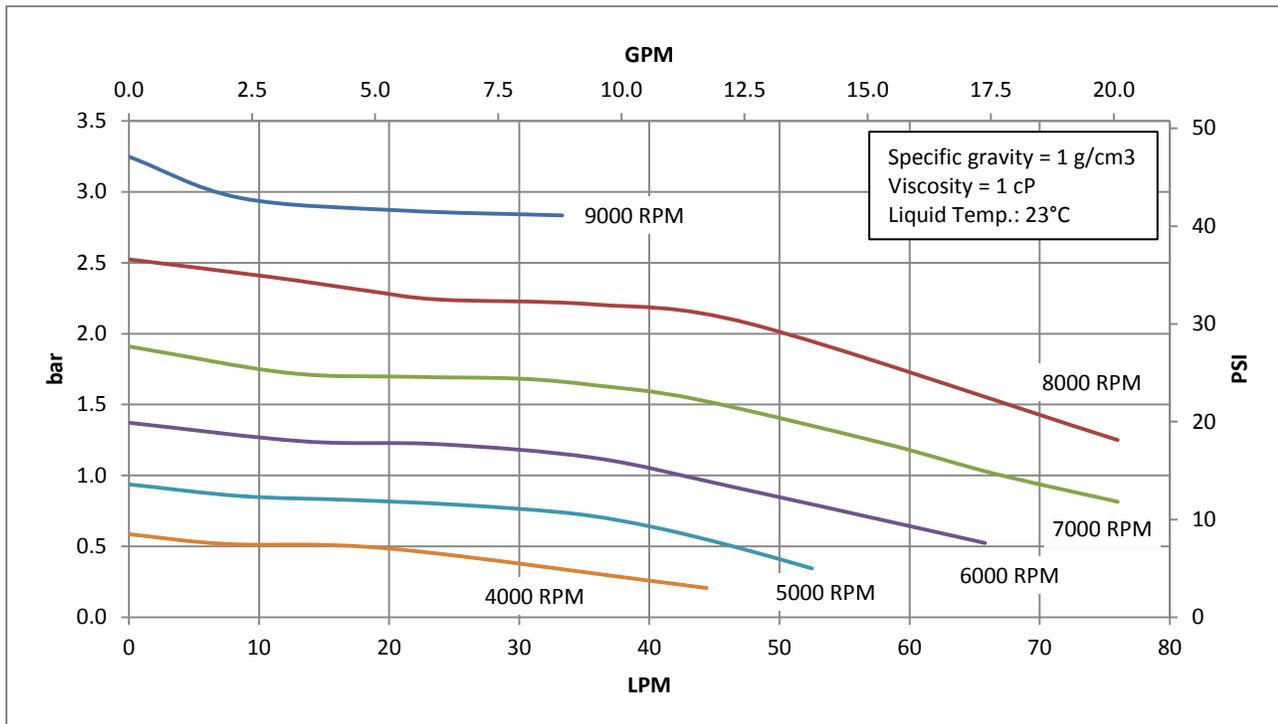
Figure 4 – Rev6 Flow vs Diff Pressure Curves
