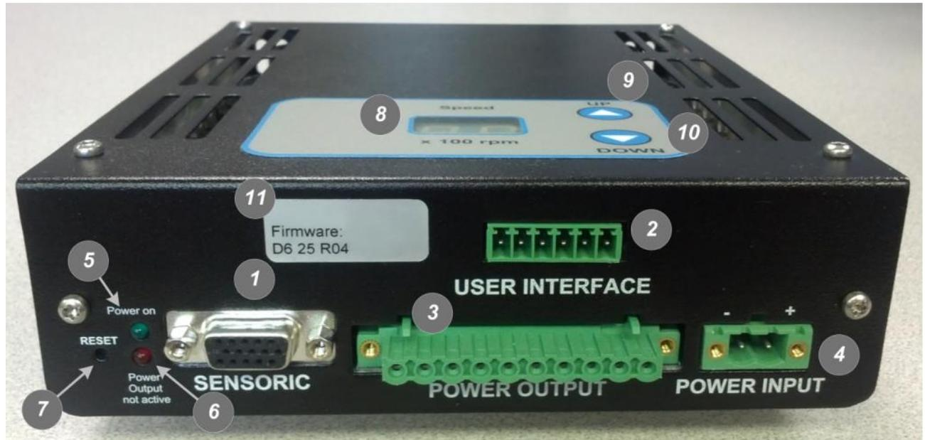
Figure 21 – Overview of the Standalone Controller Interface
