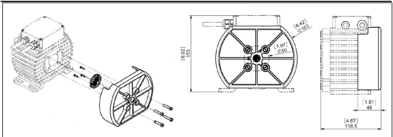
Figure 11 – Motor dimensions with attached air-cooling module.
