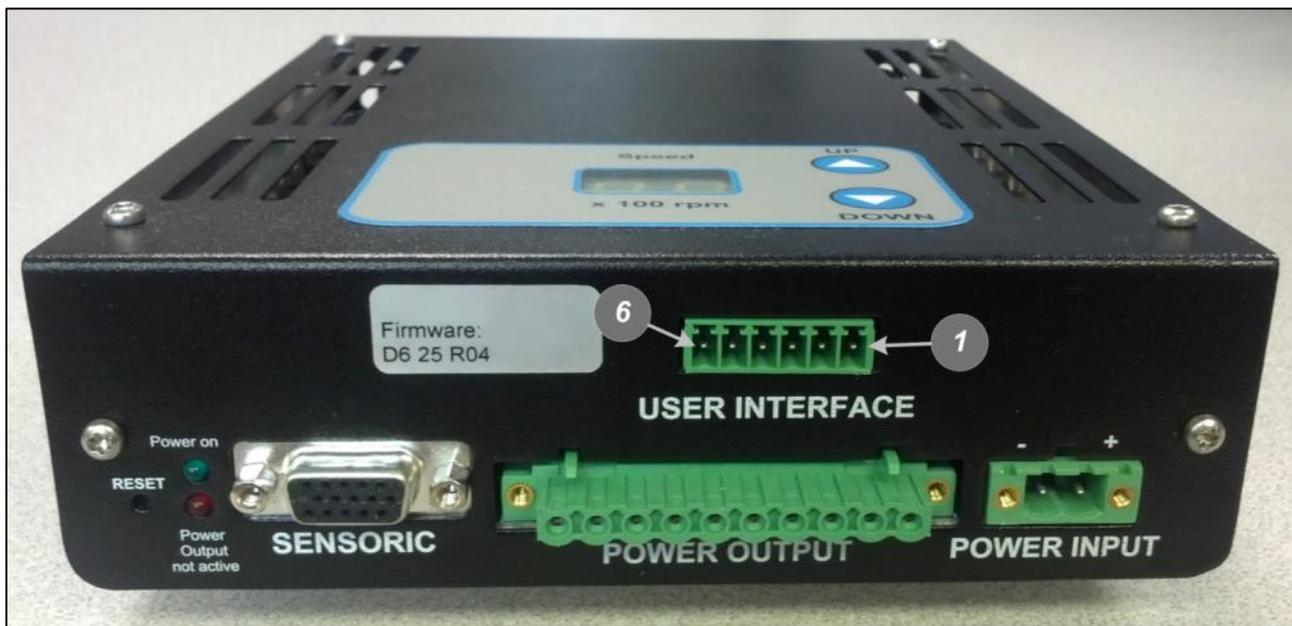
Figure 24 – “USER INTERFACE” Pin Numbering
