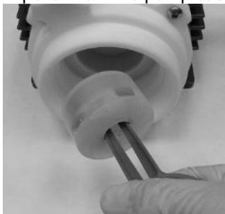
5. Inspect the wet area of the pump head carefully. In case of material damage, replace the pump casing and inlet housing.
