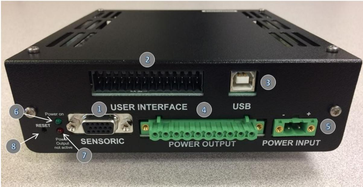
Figure 22 – Overview of the Standalone Controller Interface
