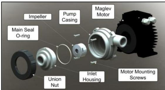
Figure 29 – Labeled Exploded View of Pump
