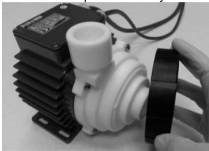
3. Loosen the fluid port adapter enough to insert the Impeller Removal Tool. Use the tool to pull the inlet housing and main seal o-ring from the pump casing.
