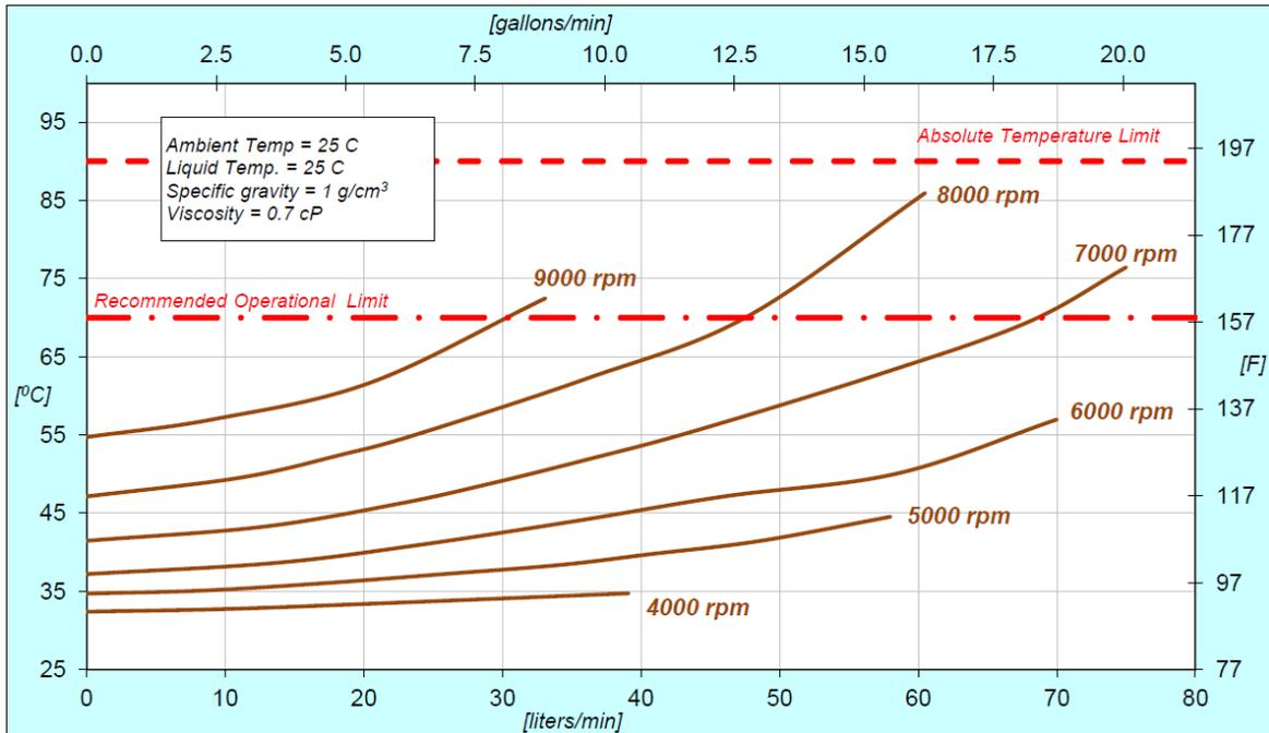
Figure 16 - Temperature Curves of the Motor for 25°C Fluid Temperature
