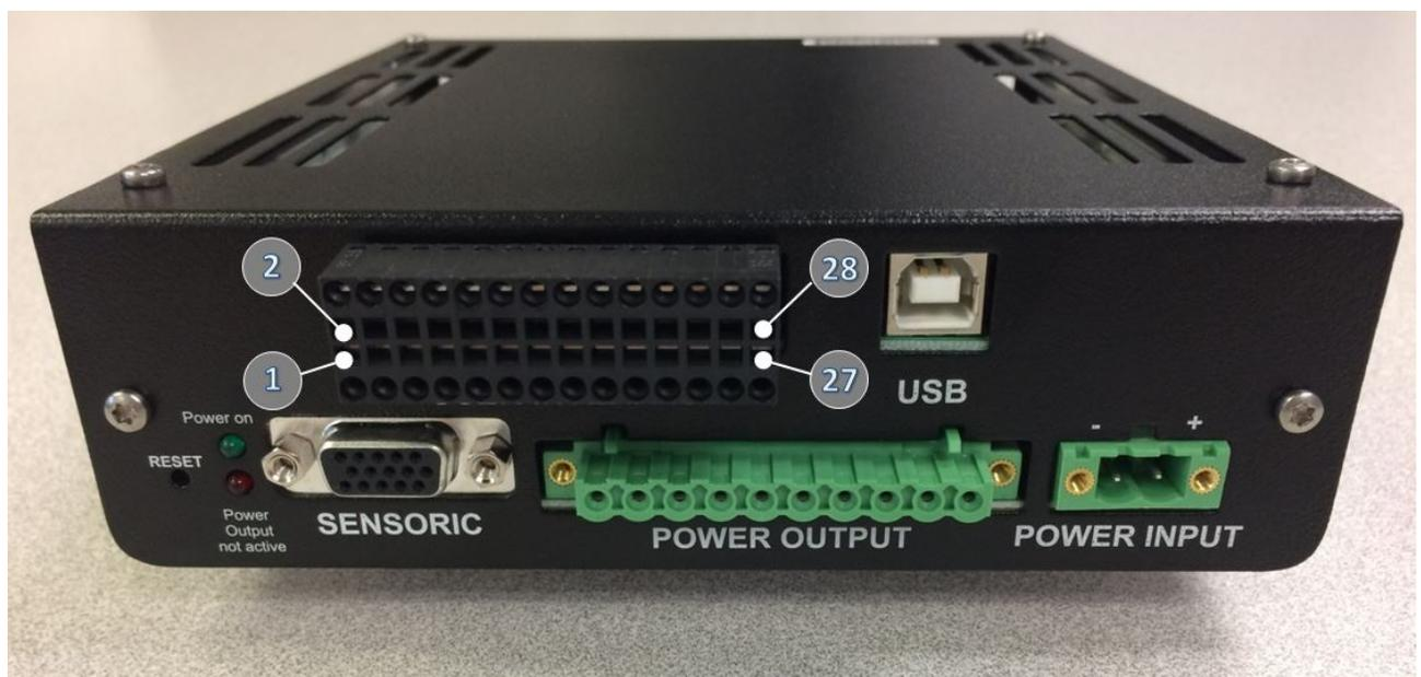
**Figure 26 – Mounted PLC connector and Pin Numbering**
