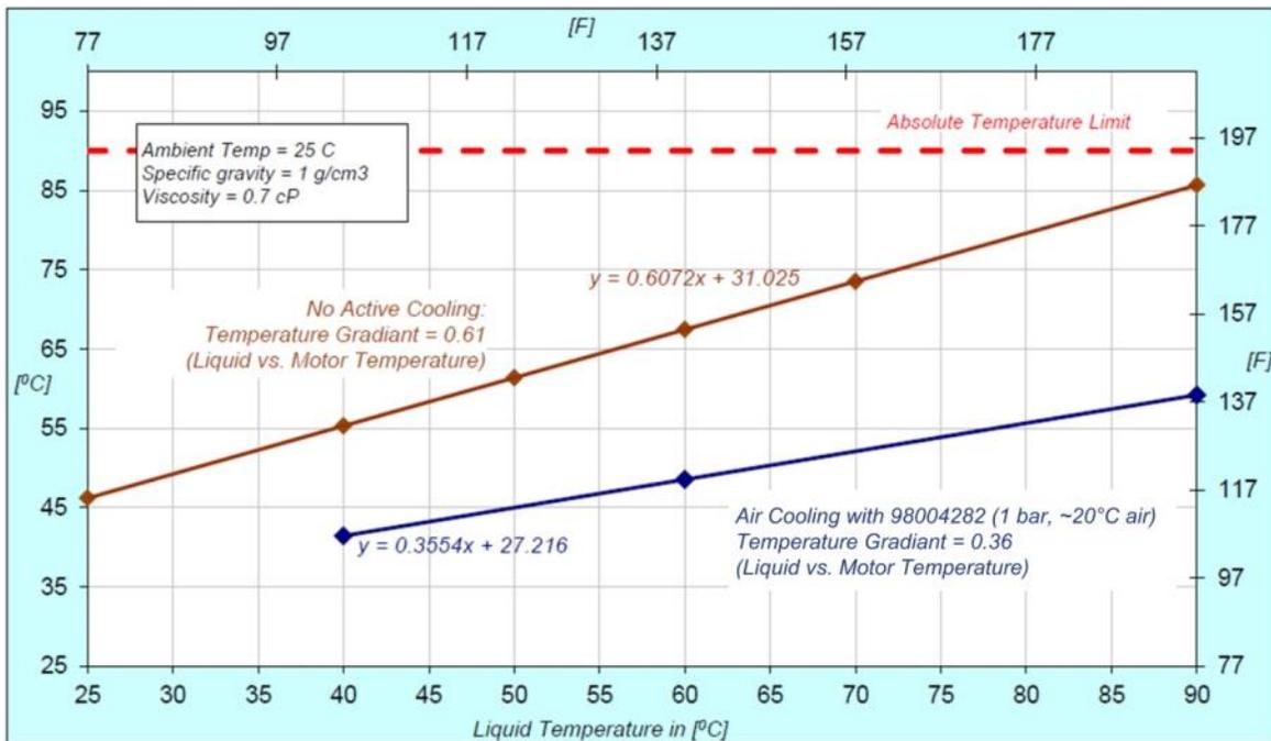
Figure 19 – Fluid Temperature Influence on Motor Temperature
