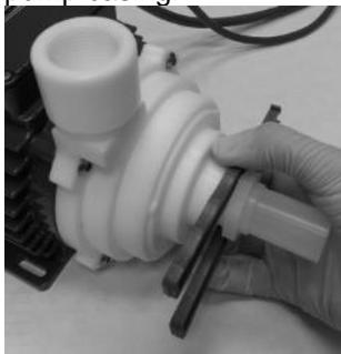
4. Gently slide the nose of the Impeller Removal Tool into the center hole of the impeller. Squeeze the handle of the tool and pull the impeller from the pump casing.
