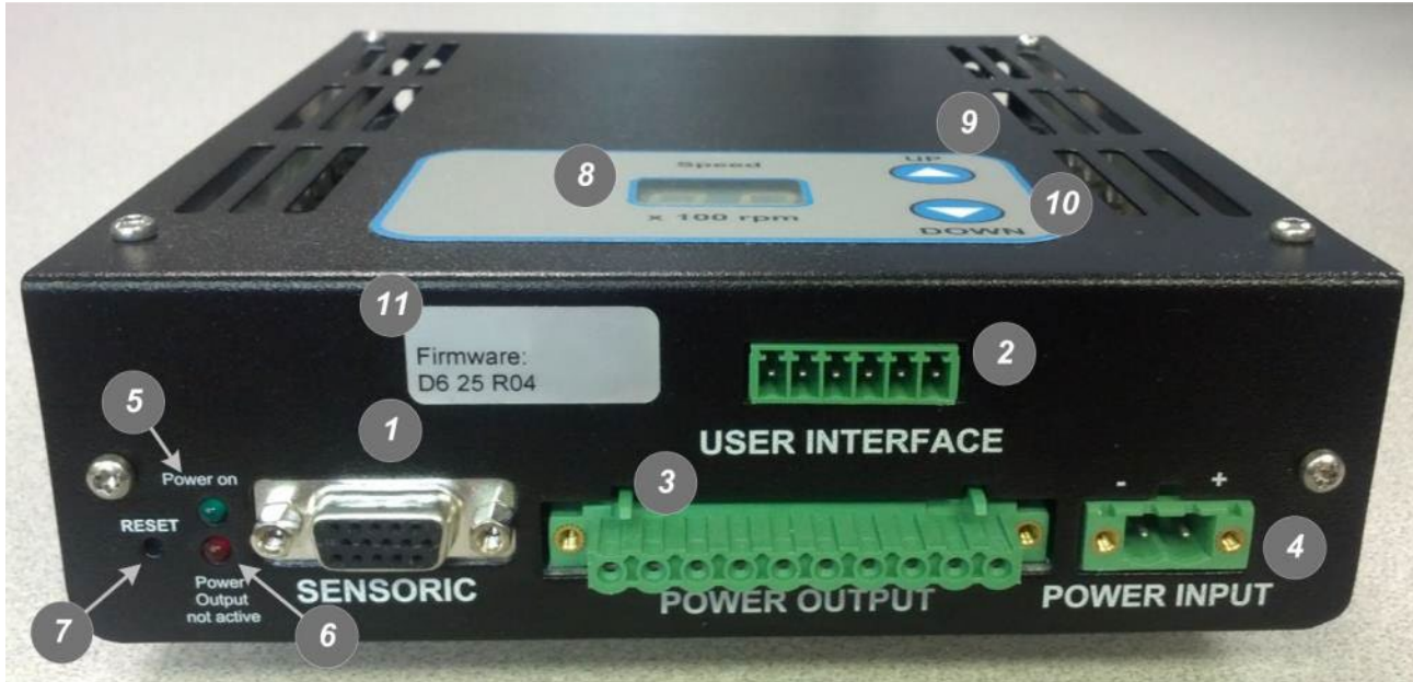
Figure 21 – Overview of the Standalone Controller Interface
