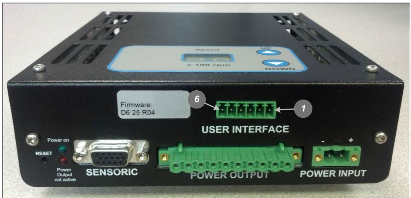
Figure 24 – “USER INTERFACE” Pin Numbering
